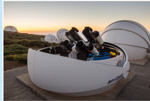
Fig.2 GOTO dome with 8 telescopes in La Palma. Image Credit: GOTO Consortium ( http://goto-observatory.org/ )
